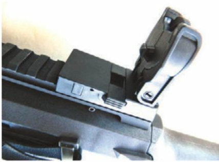
To raise sights, button is pushed from one side. To fold, button on opposite side is depressed.
