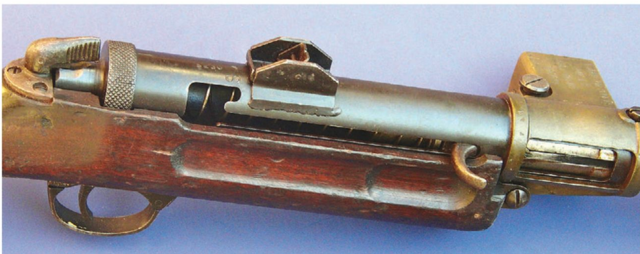
Lanchester's rear sight was protected by ears and initially quite optimistic, having a setting to 600 yards. This is the later flip-up 100/200-yard style.
