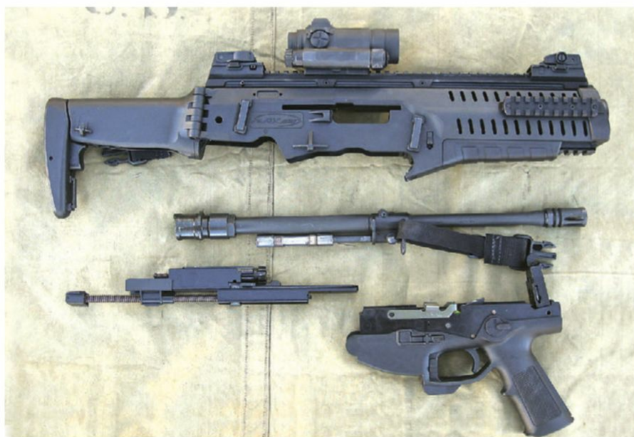
Beretta ARX can be easily and quickly disassembled into four main parts for cleaning and lubrication.
